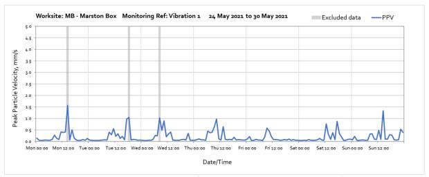
Note: High vibration levels at 14:00 on Monday 24<sup>th</sup> May and at08:00 on Wednesday 26<sup>th</sup> May are not a result of HS2 works as no works were taking place in proximity of the monitor at this time.
