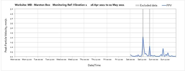
Note: High vibration levels at 13:00 and 20:00 on Saturday 1<sup>st</sup> May were outside core hours of the worksite and are not representative of HS2 vibration levels at nearby receptors.
