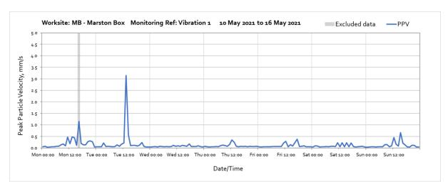
Note: High vibration levels at 16:00 on Monday 10<sup>th</sup> May are not a result of HS2 works as no works were taking place in proximity of the monitor at this time.
