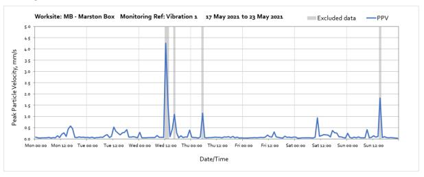
Note: High vibration levels between 12:00 and 14:00, and at 19:00 on Wednesday 19<sup>th</sup> May are not a result of HS2 works as no works were taking place in proximity of the monitor at this time.
