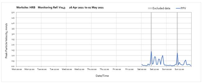
Note: Higher vibration levels measured throughout the weekend were due local intereference of the monitor and are not representative of HS2 vibration levels.
