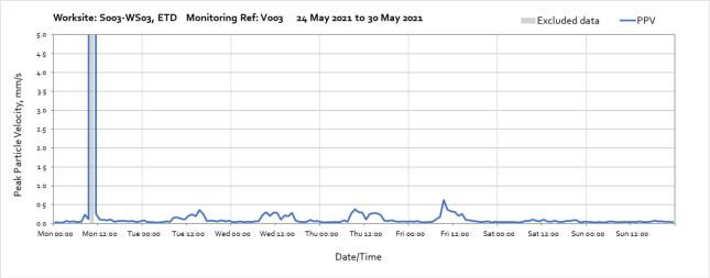
Note: High vibration levels measured between 10:00 - 11:00 on Monday  $24^{th}$  May were due to local intereference of the monitor and are not representative of HS2 vibration levels.
