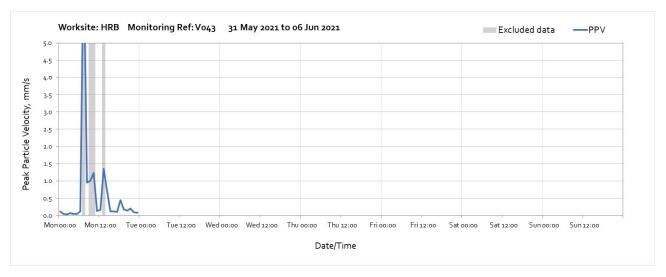
Note: High vibration levels measured throughout Monday 31st May were due to local interfernce of the monitor and are not representative of HS2 vibration levels.
