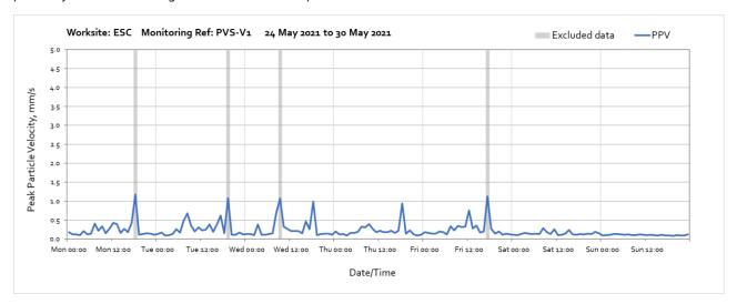
Note: Higher vibration levels measured throghout the week were due works being undertaken within close proximity of the monitoirng station and are not representative of HS2 vibration levels.
