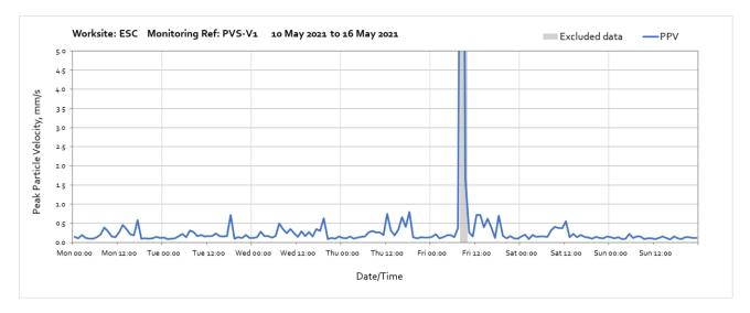
Note: High vibration levels measured between 08:00 and 10:00 on Friday 14<sup>th</sup> May were due to local intereference of the monitor and are not representative of HS2 vibration levels.
