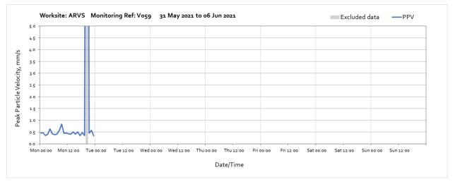
Note: High vibration levels measured between 20:00 and 21:00 on Monday 31st May were due to local intereference of the monitor and are not representative of HS2 vibration levels.
