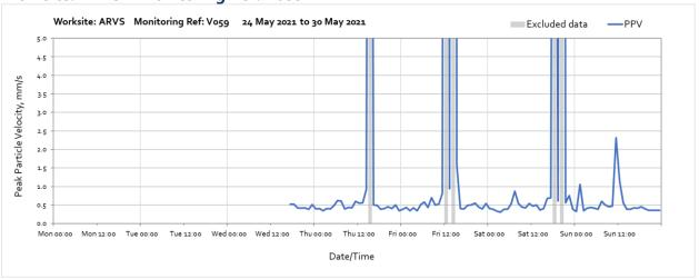
Note: Monitor was installed at 17:00 on Wednesday 26<sup>th</sup> May. High vibration levels measured throughout the week were due to local intereference of the monitor and are not representative of HS2 vibration levels.
