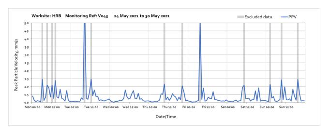
Note: High vibration levels measured throughout the week were due local intereference of the monitor and are not representative of HS2 vibration levels.
