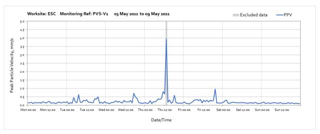
Note: High vibration levels measured between 13:00 and 14:00 on Thursday 6<sup>th</sup> May were due to local intereference of the monitor and are not representative of HS2 vibration levels.
