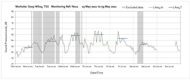
Note: Missing data from 00:00 until 18:00 on Sunday 9<sup>th</sup> May was due to a fault with the monitoring station. The monitoring station has been replaced with view of minimising further loss of data.
