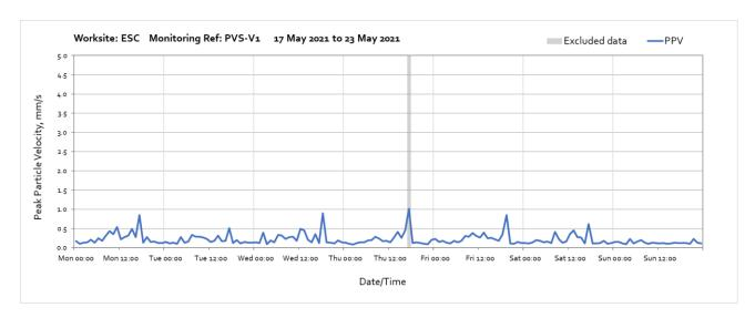
Note: Higher vibration levels measured between 17:00 and 18:00 were due works being undertaken within close proximity of the monitoiring station and are not representative of HS2 vibration levels.
