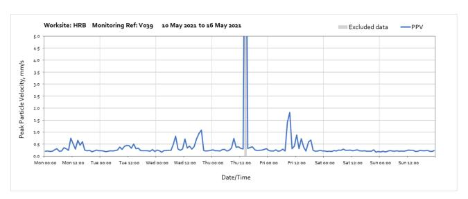
Note: High vibration levels measured at 14:00 on Thursday 13<sup>th</sup> May were due to local interference of the monitor and are not representative of HS2 vibration levels.
