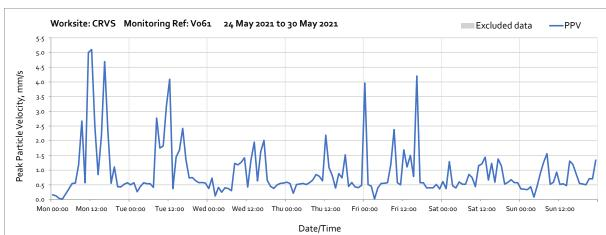
Note: Vibration monitor was installed at 11:00 on the 20th of May.
