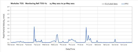
Note: High vibration at 08:00 on Tuesday 25<sup>th</sup> May; at 16:00 on Wednesday 26<sup>th</sup> May, at 08:00 and at 11:00 on Friday 28<sup>th</sup> May were to the tracking of vehicles on the internal haul road nearby the vibration monitor and are not representative of HS2 vibration levels at nearby receptors.
