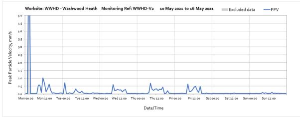
Note: High vibration levels at 02:00 on Monday 10<sup>th</sup> May were due to local interference of the monitor and are not representative of HS2 vibration levels at nearby receptors.
