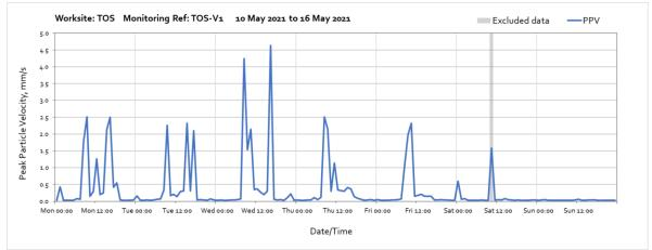
Note: High vibration levels measured aboe 1mm/s were due to the tracking of vehicles on the internal haul road nearby the vibration monitor and are not representative of HS2 vibration levels at nearby receptors.
