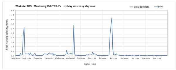
Note: High vibration levels at 08:00 and 10:00 on Monday 17<sup>th</sup> May; at 16:00 on Wednesday 19<sup>th</sup> May and between 07:00 - 11:00 on Friday 21<sup>st</sup> May were due to the tracking of vehicles on the internal haul road nearby the vibration monitor and are not representative of HS2 vibration levels at nearby receptors.
