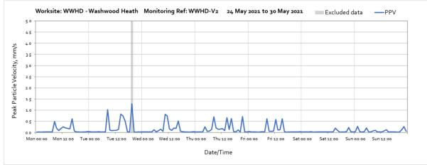
Note: High vibration levels at 19:00 on Tuesday 25<sup>th</sup> May were due to loccal interference of the monitor and are not representative of HS2 vibration levels at nearby receptors.
