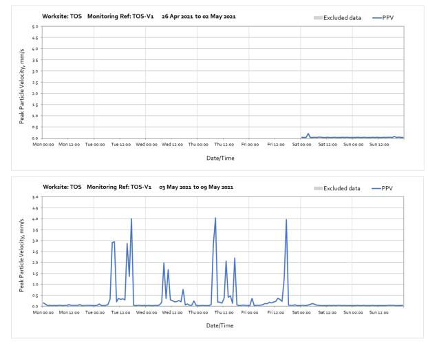
Note: High vibration levels measured above 1mm/s were due to the tracking of vehicles on the internal haul road nearby the vibration monitor and are not representative of HS2 vibration levels at nearby receptors.
