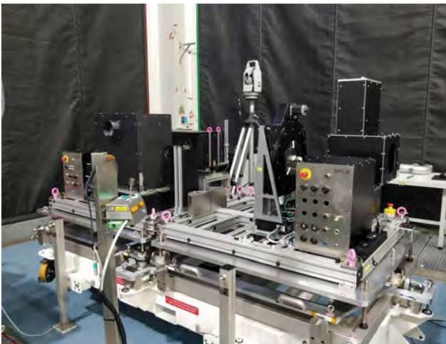
OGSE, delivered by NPL, will be used to characterise and calibrate the MicroCarb CO 2 Measurement Instrument on the ground. The final two images show the front of the telescope, part of OGSE, set up at NPL.
