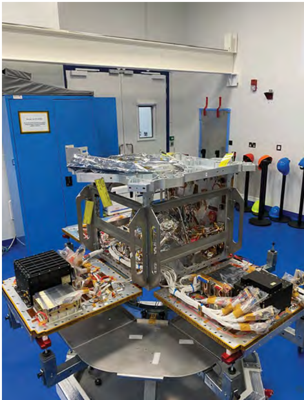
PCS delivered by RAL Space, and used to support MicroCarb CO 2 measurement instrument calibration and targeted local measurements in orbit.
