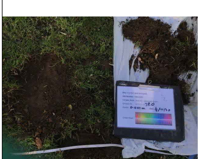
Photo 2: Excavated soil ready for sampling
