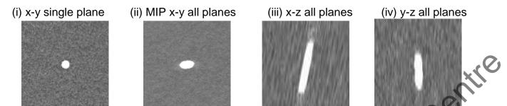
Figure 11. Extracts from planes showing 1mm aluminium ball in (i) single focal plane, (ii) Maximum Image Projection (MIP) through all focal planes, and through re-sliced vertical planes in the directions (iii) parallel and (iv) perpendicular to the chest wall?
