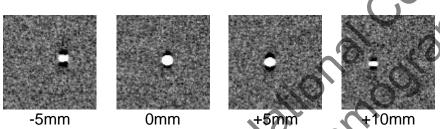
Figure 10. Appearance of 1mm aluminium balls in reconstructed slabs at 5mm intervals, from 5mm below to 10mm above the slab of best focus
