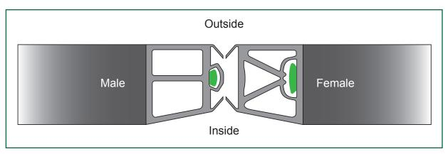
*Figure 9: Cross–section through the sensitive door edges, showing the rubber sealing edge profiles housing the electrical sensing elements (shown in green)*
