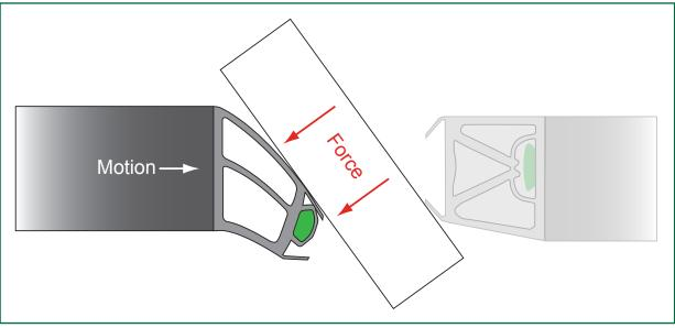
*Figure 11: Cross* –section through the sensitive door edges, showing the rubber sealing edge profiles and the deflected male edge
