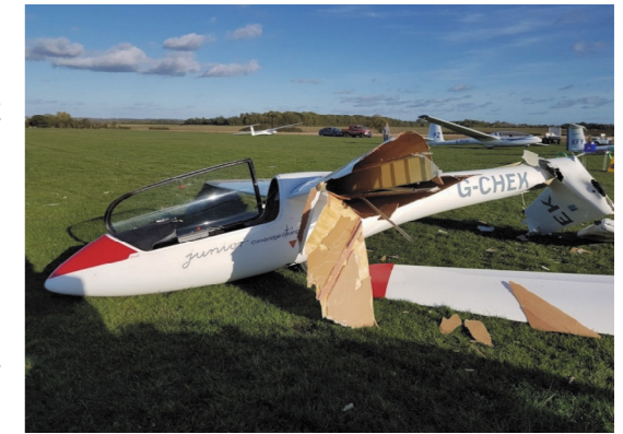
Damage to the tail and left wing of an SZD-51 glider caused by G-ROYC
