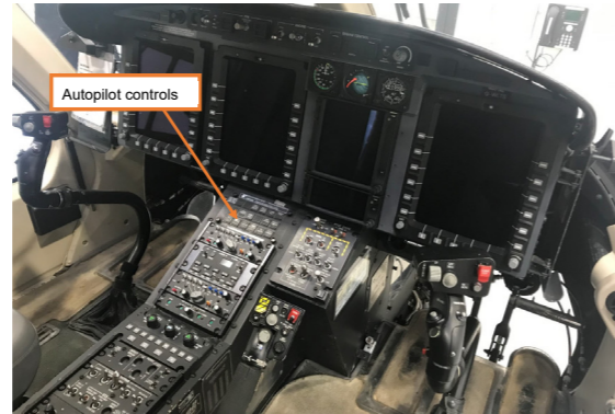
Autopilot control panel
