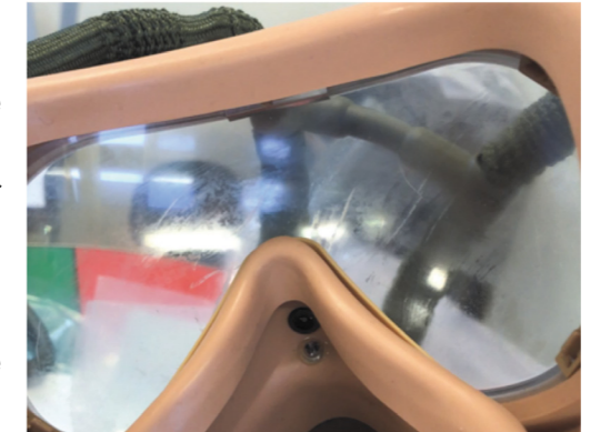
Co-pilot's mask showing fogging and marks on internal lens
