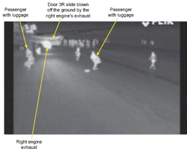
RFFS infrared CCTV showing some passengers leaving with baggage
