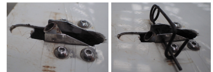
Locking lever when tailplane attached (left image) and when locked with safety pin inserted (right image)
