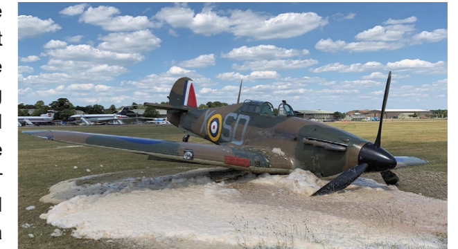
G-HRLI after the accident and application of fire-suppressing agent
