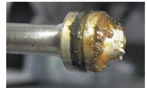
Material adjacent to tie bar fracture surface
