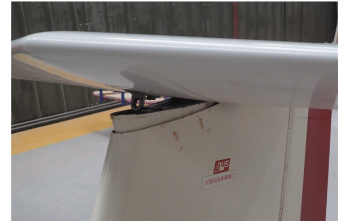
Rear tailplane mechanism partially engaged, front fitting disengaged
