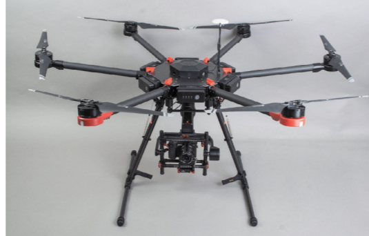
M600 series aircraft The accident aircraft was fitted with three GPS antenna
