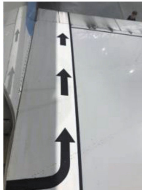
Overwing exit escape route markings on E195 (view towards wing trailing edge)
