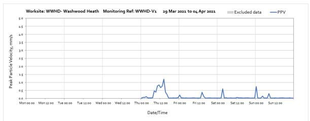
Note: High vibration levels at 14:00 on Thursday  $1^{st}$  April were due to tracking plant nearby the vibration monitor and are not representative of HS2 vibration levels at nearby receptors.
