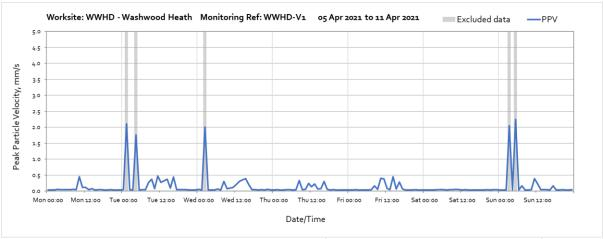
Note: High vibration levels at 01:00 and 04:00 on Tuesday 6<sup>th</sup> of April, and at 02:00 on Wednesday 7<sup>th</sup> April, were outside of HS2 work hours and due to local interference and are not representative of HS2 vibration levels.
