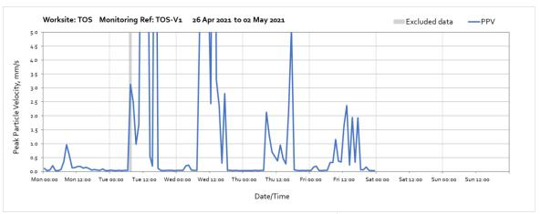
Note: High vibration levels between 07:00 and 17:00 on Tuesday 27<sup>th</sup> April were due to construction of the haul road, including stabilisation works, placement of fill and compaction immediately adjacent (within 2m) to the vibration monitor and are not representative of HS2 vibration levels at nearby receptors.
