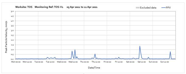
Note: High vibration level at 10:00 on Saturday  $10^{th}$  April was due tracking plant nearby the vibration monitor and are not representative of HS2 vibration levels at nearby receptors.
