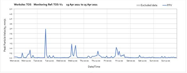
Note: High vibration levels at 08:00 on Wednesday 20<sup>th</sup> April, at 11:00 and at 15:00 on Wednesday 21<sup>st</sup> April, and at 09:00 on 23<sup>rd</sup> April were due tracking plant nearby the vibration monitor and are not representative of HS2 vibration levels at nearby receptors.
