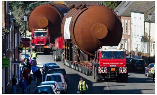
Under LLWR's landmark Berkeley Boilers project, 2012/13, 15 redundant 300 tonne steel boilers, each 22m long, were transported four miles through Berkeley town centre and on to the coast for shipping to Sweden. Around 95% of the steel was recycled for reuse.
