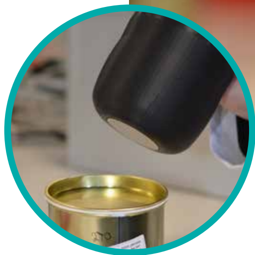
An example of technology under development for POCO is gamma-optical video imaging (GOVI), a handheld camera that can be deployed through 6" ports. It provides real time visualisation and the location of gamma activity and could simplify the glovebox POCO process (Images courtesy of Loughborough University)
