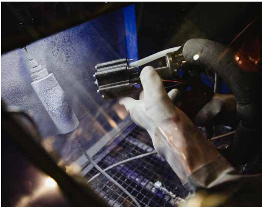
Rawwater's molten metal manipulation (M 3 ), a crack repair system that can be used to provide high integrity seals in ponds, vessels and pipes
