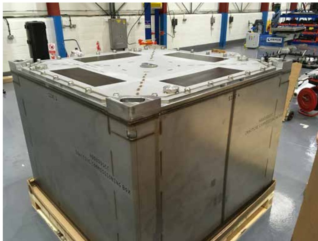
An example of a container used on the Sellafield site to store nuclear waste
