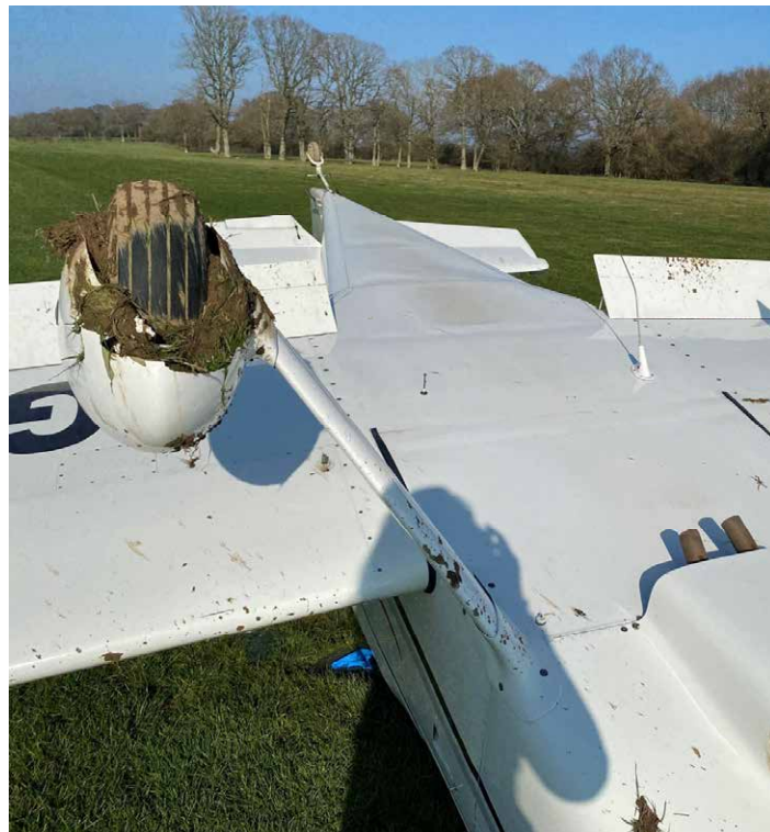
Figure 2 Contamination and damage to one of the wheel spats (pictures courtesy of the pilot)
