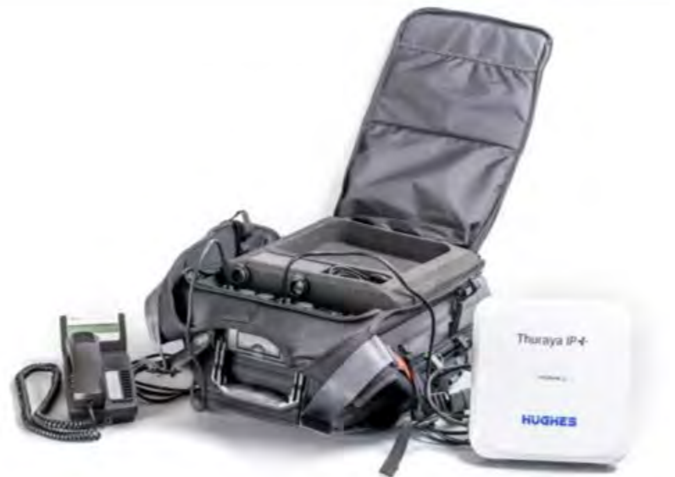
Figure 50: SCYTALE satellite communications equipment
