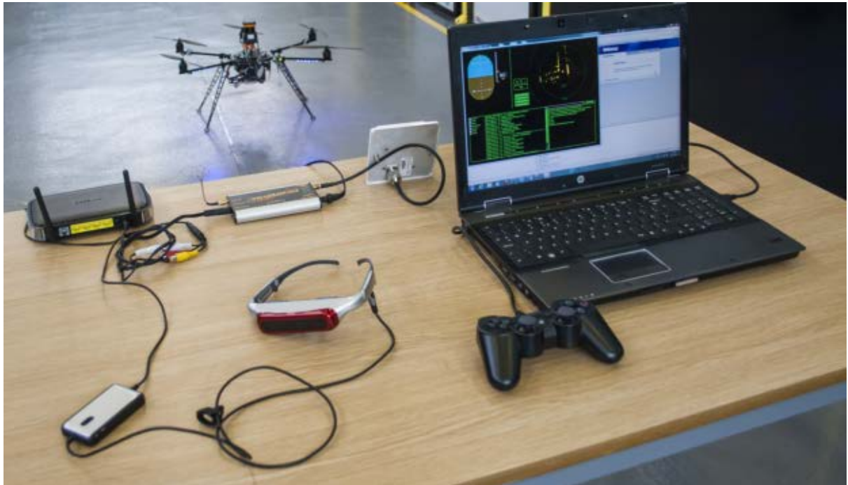
Figure A5: UAV base-station. [3]
