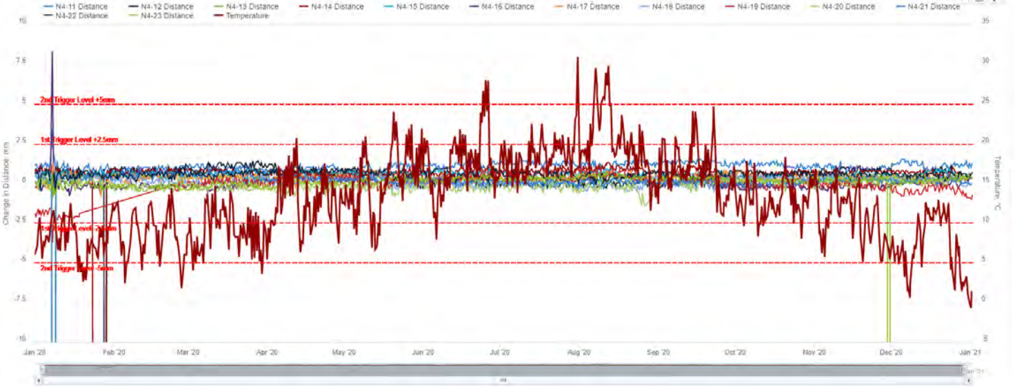
N5 Laser Distometers vs Temperature - Last Year
