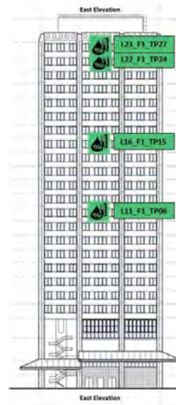
Temperature & Humidity Sensors Locations - East Elevation
