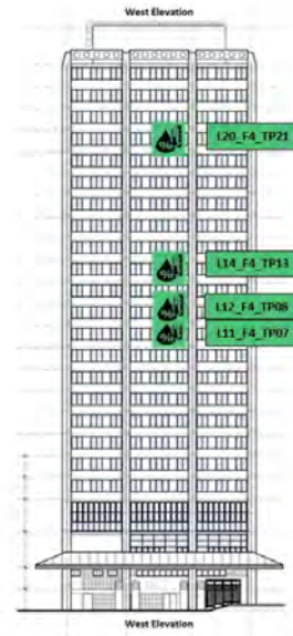
Temperature & Humidity Sensors Locations - West Elevation
