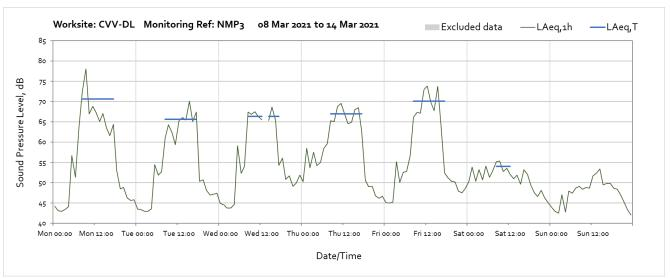
Note: Missing data at 13:00 on Wednesday 10<sup>th</sup> March 2021 was due to filed calibration of the noise monitor.
