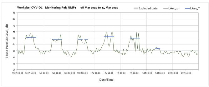
Note: Missing data at 13:00 on Wednesday 10<sup>th</sup> March 2021 was due to field calibration of the noise monitor.
