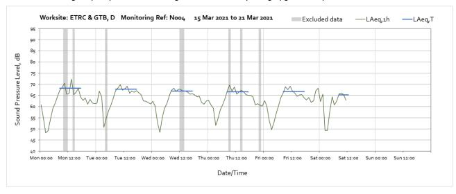
Note: Missing data from 12:00 on Saturday 20<sup>th</sup> March until 00:00 on Monday 22<sup>nd</sup> March was due to internal memory space becoming full. The internal storage capacity of the monitoring station is currently being upgraded to prevent further data loss.
