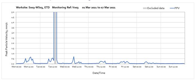
Note: High vibration levels measured between 13:00 - 15:00 on Tuesday  $2^{nd}$  March was due to local interference of the monitor and are not representative of HS2 vibration levels.
