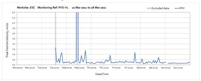
Note: Monitor was installed at 13:00 on Tuesday 23<sup>rd</sup> March. High vibration levels at 13:00 on Tuesday 23<sup>rd</sup> March were due to the setup of the monitoring station. High vibration levels measured between 10:00 on Wednesday 24<sup>th</sup> March was due to local interference of the monitor and are not representative of HS2 vibration levels. Missing data between 01:00 and 02:00 on Sunday 28th March was due to the clock change (start of BST).
