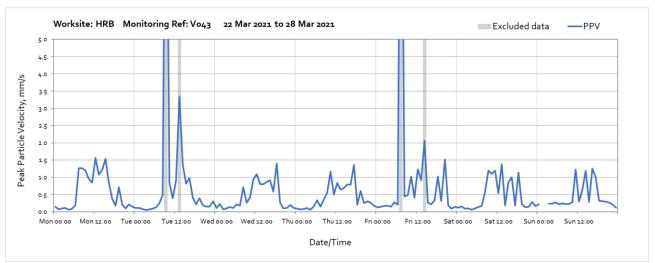
Note: High vibration levels measured throughout the week were due to the use of the neraby residential bin store and local interference of the monitor and are not representative of HS2 vibration levels. Missing data between 01:00 and 03:00 on Sunday 28th March was due to the clock change (start of BST).
