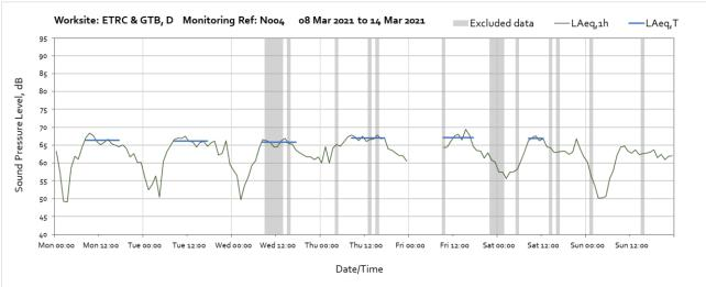
Note: Missing data from 00:00 until 09:00 on Friday 12<sup>th</sup> March was due to internal memory space becoming full. The internal storage capacity of the monitoring station is currently being upgraded to prevent further data loss.
