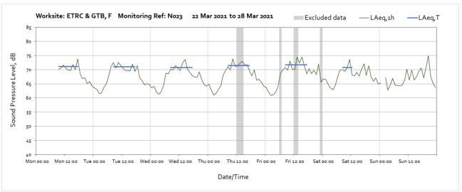
Note: Missing data from 00:00 untill 09:00 on Monday 22<sup>nd</sup> March was due to internal memory space becoming full. The internal storage capacity of the monitoring station is currently being upgraded to prevent further data loss. Missing data between 01:00 and 02:00 on Sunday 28th March was due to the clock change (start of BST).
