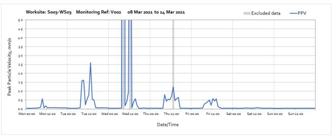
Note: High vibration levels at 08:00 and 12:00 on Wednesday  $10^{th}$  March were due to local interference of the monitor and are not representative of HS2 vibration levels. High vibration levels at 12:00 on Thursday  $11^{th}$  March were due to routine maintenance of the monitoring station.
