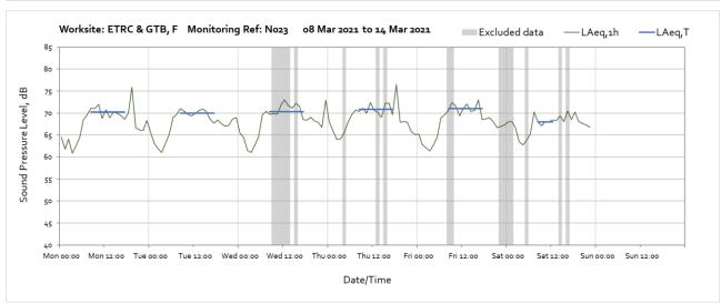
Note: Missing data from 23:00 on Saturday 13<sup>th</sup> March until 00:00 on Monday 15<sup>th</sup> March was due to internal memory space becoming full. The internal storage capacity of the monitoring station is currently being upgraded to prevent further data loss.
