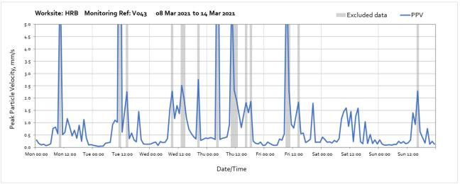
Note: High vibration levels measured throughout the week were due to the use of the neraby residential bin store and local interference of the monitor and are not representative of HS2 vibration levels.
