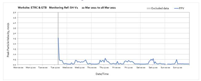
Note: Monitor was installed at 15:00 on Tuesday 23<sup>rd</sup> March. High vibration levels at 15:00 on Tuesday 23<sup>rd</sup> March were due to the setup of the monitoring station and are not representative of HS2 vibration levels. Missing data between 01:00 and 02:00 on Sunday 28th March was due to the clock change (start of BST).
