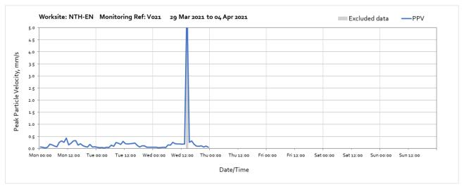
Note: High vibration levels at 14:00 on Wednesday 31<sup>st</sup> March were due to routine maintenance of the monitoring station and are not representative of HS2 vibration levels.
