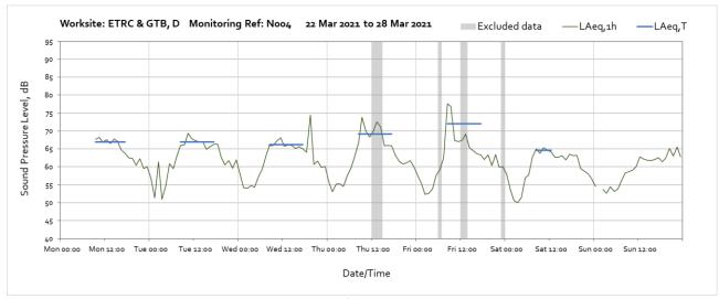
Note: Missing data from 00:00 until 09:00 on Monday 22<sup>nd</sup> was due to internal memory space becoming full. The internal storage capacity of the monitoring station is currently being upgraded to prevent further data loss. Missing data between 01:00 and 02:00 on Sunday 28th March was due to the clock change (start of BST).
