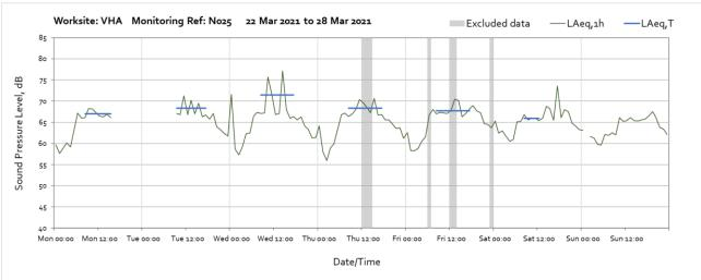
Note: Missing data from 16:00 Monday 22<sup>nd</sup> March untill 09:00 on Monday 23<sup>rd</sup> March was due to internal memory space becoming full. The internal storage capacity of the monitoring station is currently being upgraded to prevent further data loss. Missing data between 01:00 and 02:00 on Sunday 28th March was due to the clock change (start of BST).
