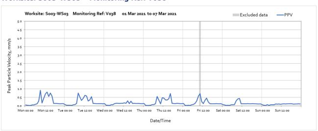
Note: High vibration levels at 10:00 on Friday  $5^{th}$  March were due to routine maintenance of the monitoring station and are not representative of HS2 vibration levels.
