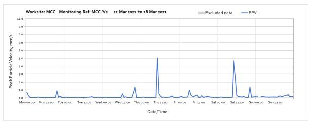
Note: No construction activities were undertaken in the month, measured vibration levels representative of ambient vibrations without contribution from HS2. Missing data at 02:00 on Sunday 28th March 2021 was due to the clocks going forward at the start of British Summer Time.
