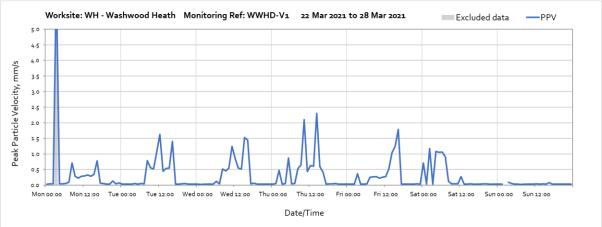
Note: High vibration levels at 03:00 on Monday the 22<sup>nd</sup> of March were outside of HS2 work hours and due to local interference and are not representative of HS2 vibration levels. Missing data at 02:00 on Sunday 28th March 2021 was due to the clocks going forward at the start of British Summer Time.
