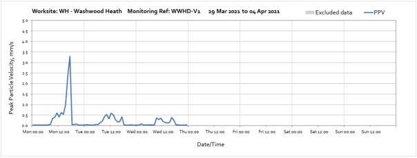
Note: High vibration levels between 16:00 and 18:00 on Monday the 29<sup>th</sup> of March were due to trial holes being undertaken near the monitor and are not representative of HS2 vibration levels at the receptor location.
