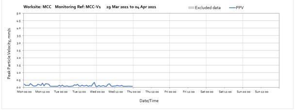
Note: No construction activities were undertaken in the month, measured vibration levels representative of ambient vibrations without contribution from HS2.
