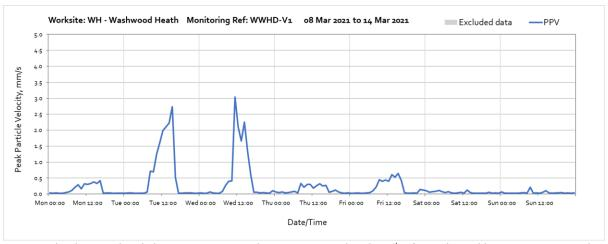
Note: High vibration levels between 10:00 and 16:00 on Tuesday the 9<sup>th</sup> of March, and between 11:00 and 16:00 on Wednesday 10<sup>th</sup> of March were due to haul road costruction being undertaken at close proximity to the vibration monitor and are not representative of HS2 vibration levels at nearby receptors.
