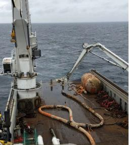
Figure 9.5: SAL buoy and loading hose retrieved to AHV deck
