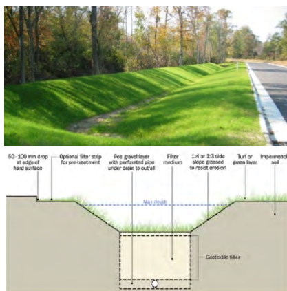
Figure 17.2: Typical dry swale
