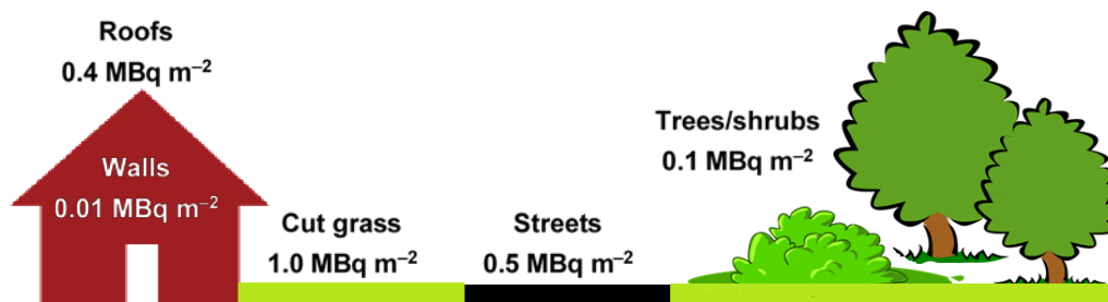
Figure 3.2 Contamination levels of ^{137}\text{Cs} on the various types of surface in the city for the hypothetical scenario. The diagram shows deposition ( \text{MBq m}^{-2} ) of ^{137}\text{Cs} on a range of surfaces for a hypothetical scenario involving an atmospheric release of radionuclides to an inhabited area. Highest levels of deposition are to horizontal soil and grassed areas ( 1.0 \text{ MBq m}^{-2} ). Conversely, lowest levels of deposition are to vertical surfaces such as walls ( 0.01 \text{ MBq m}^{-2} ).
