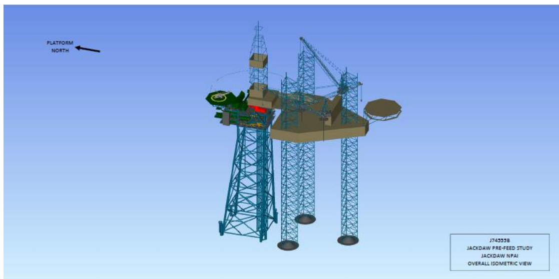
Figure 2-7 Example WHP view with Jack-up on station.
