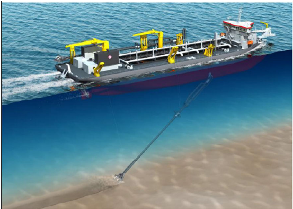
Figure 2-9 Trailing suction hopper dredger
