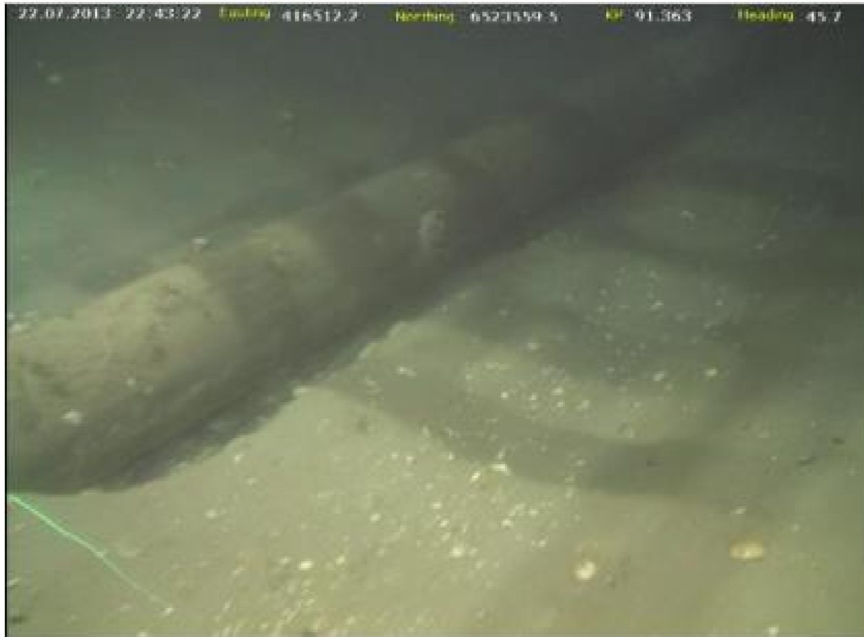
Figure C-3 Image from 2013 pipeline survey at KP 91.363 showing section of PL301 exposure within the trench
