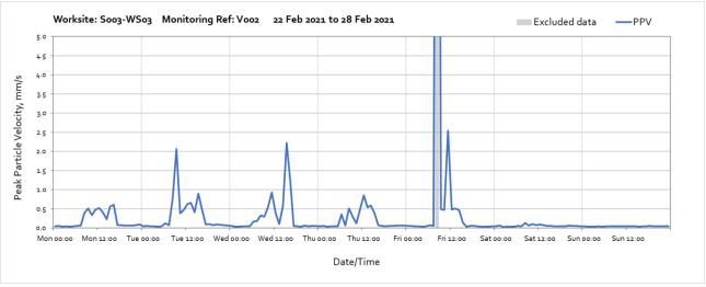
Note: High vibration levels measured at 08:00 on Friday 26<sup>th</sup> February were due to local interference of the monitor and are not representative of HS2 vibration levels.
