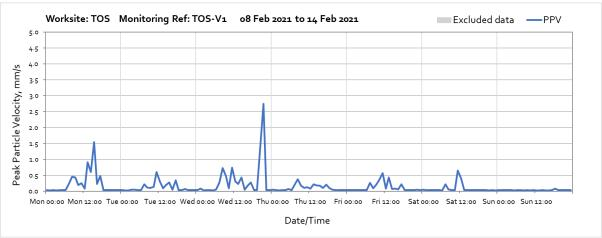
Note: High vibration levels at various time of the week were due to the soil stripping and ground stabilisation activity undertaken at close proximity to the vibration monitor and are not representative of HS2 vibration levels at nearby receptors .
