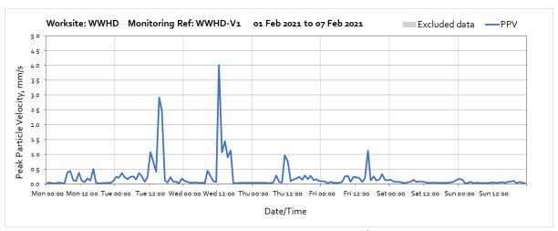
Note: High vibration levels between 15:00 and 16:00 on Tuesday the 2<sup>nd</sup> of February, and between 12:00 and 16:00 on Wednesday 3<sup>rd</sup> of February were due to the construction of safety bunds at close proximity to the vibration monitor and are not representative of HS2 vibration levels at nearby receptors.
