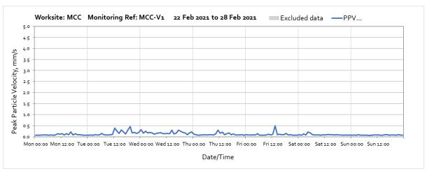
Note: No construction activities were undertaken in the month, measured vibration levels representative of ambient vibrations without contribution from HS2.
