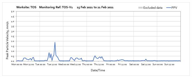
Note: High vibration levels at various time of the week were due to the soil stripping and ground
