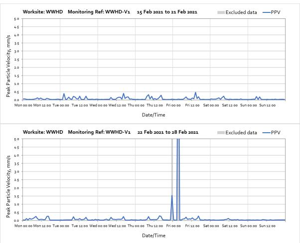
Note: High vibration levels at 23:00 on Thursday the 25<sup>th</sup> of Februray and 03:00 on Friday the 26<sup>th</sup> of February were outside of HS2 work hours and caused due to local interference and are not representative of HS2 vibration levels.
