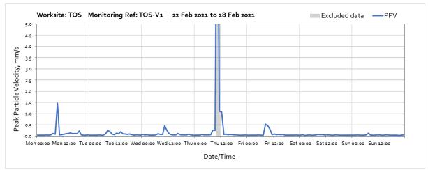
Note: High vibration levels at 10:00 on Thursday the 25<sup>th</sup> of February were due to the disturbance caused from the relocation of the monitor and are not representative of HS2 vibration levels.
