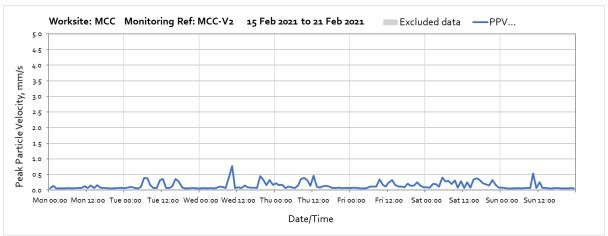
Note: No construction activities were undertaken in the month, measured vibration levels representative of ambient vibrations without contribution from HS2.
