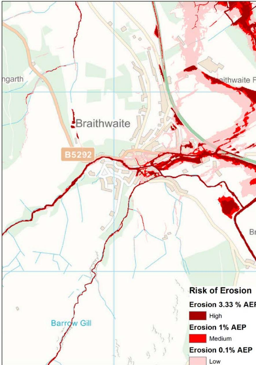
Figure 4.2 Risk of erosion map for scenario 1:  $n = 0.05$ ;  $D50 = 0.08$  m
