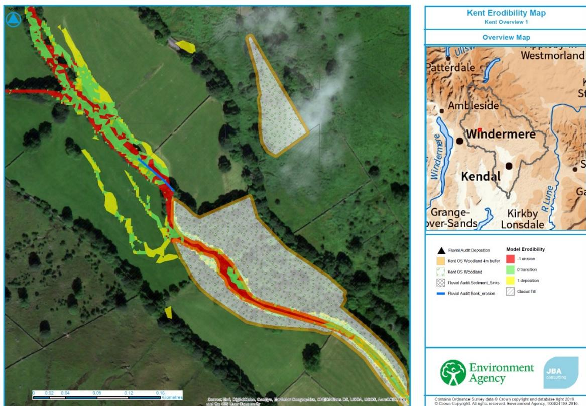
Figure 5-3 Kent - Improvement 2 - removing areas of high shear in areas of existing woodland
