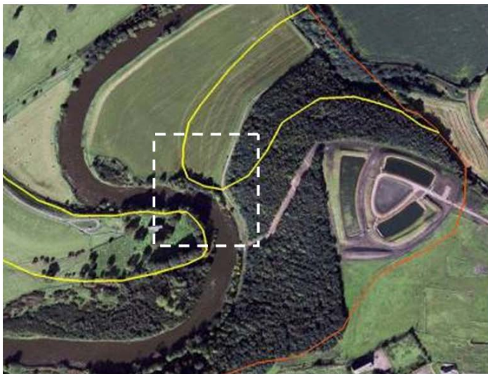
Constriction due to Natural processes (e.g. Glacial features constrict the channel and floodplain flows).
