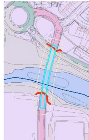
Constriction due to Human modification (e.g. Road bridge).
