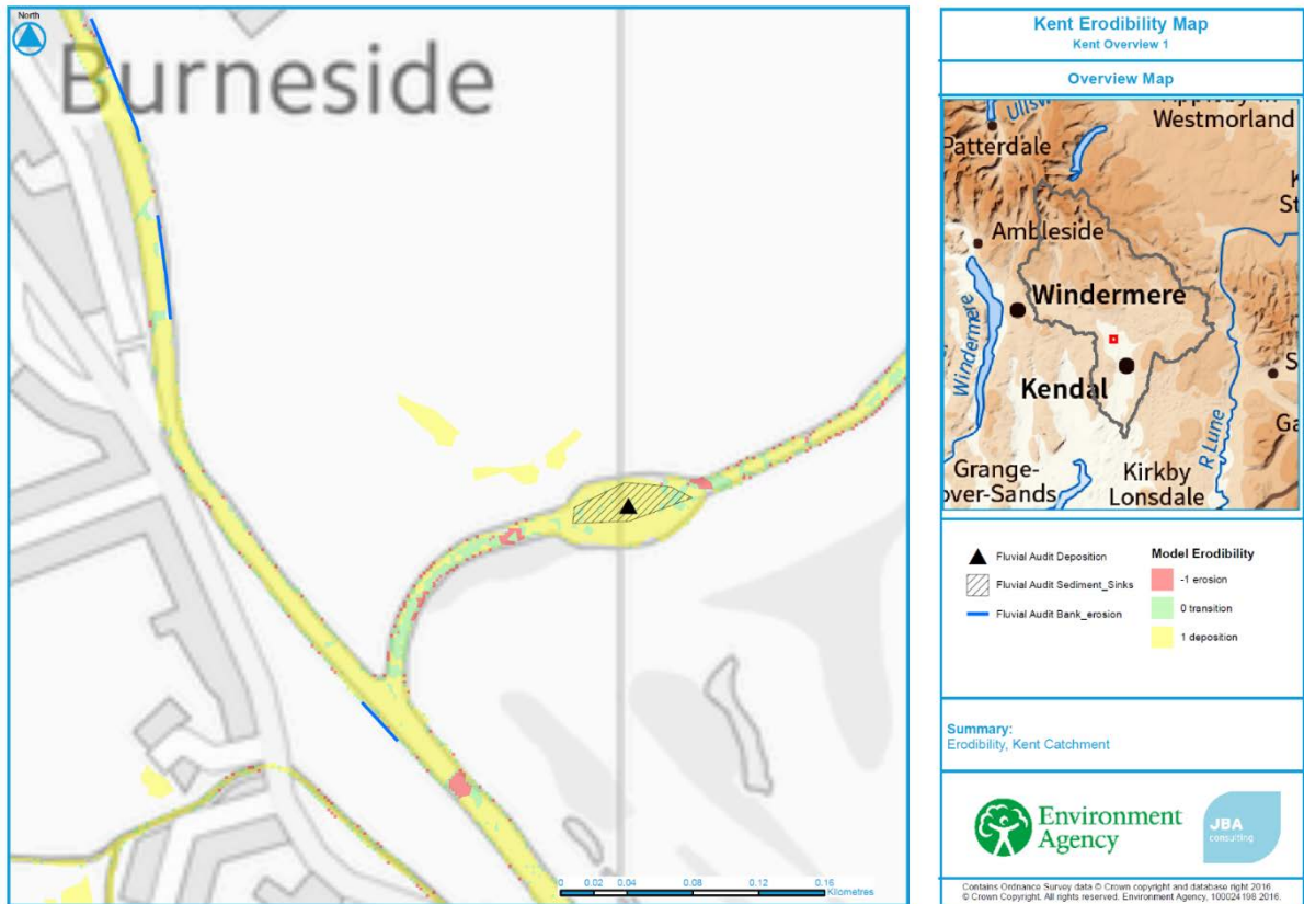
Figure D-29 Kent - Depositional areas identified correctly, with some areas of bank erosion downstream of Burneside
