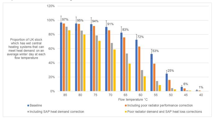
Figure 3 - The proportion of UK dwellings, with wet central heating systems, that could meet heat demand (kW) on a typical winter day at each flow temperature. (Average temperature across sample is 4.7°C, error bars give the 95% confidence interval)
