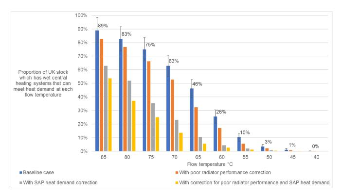
Figure 2- Proportion of UK dwellings, with wet central heating systems, that could meet peak heat demand (kW) at each flow temperature. (Average temperature across sample for the peak is -3.5°C. Error bars give 95% statistical confidence interval.
