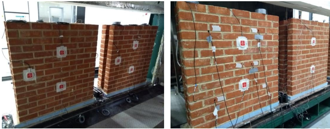
Figure 1 Cavity wall specimens instrumentation towards the external (left) and indoor (right) simulated environments.
