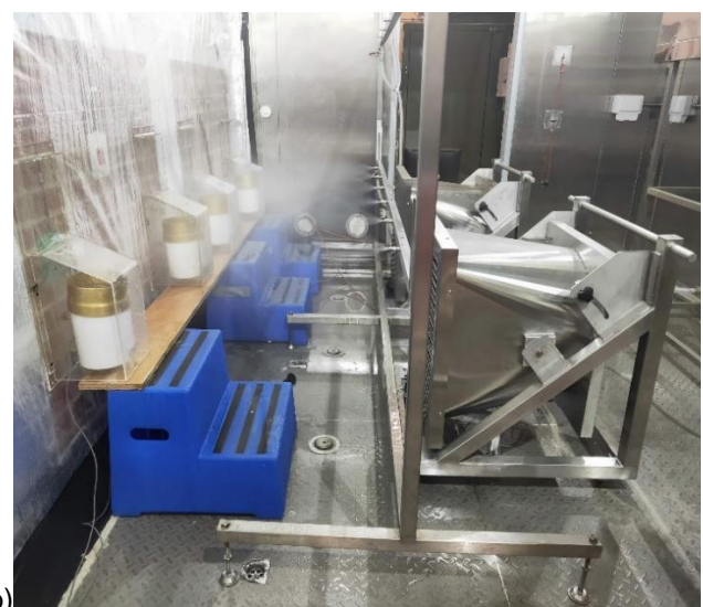
Figure 8: a) Theoretical patterns of wetting of walls during WDR tests b) Calibration of water distribution with WDR gauges
