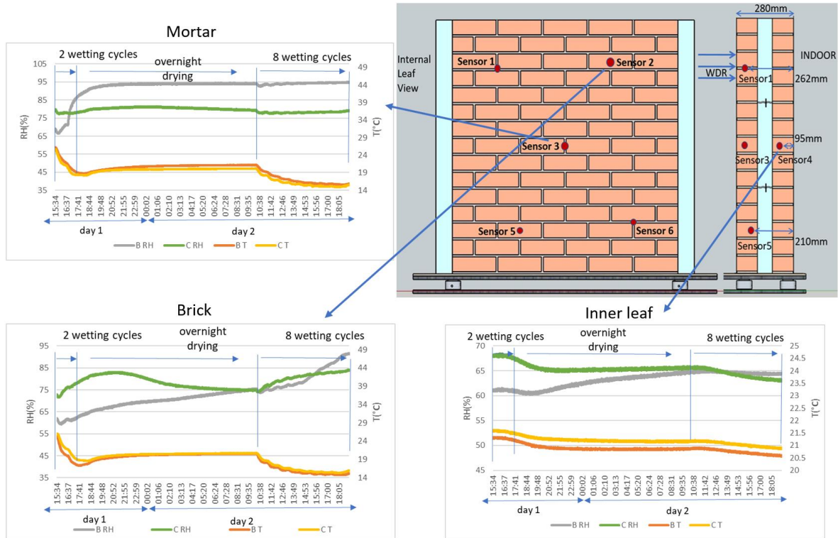
Figure 17: Variation of in wall temperature and RH for the B2 and C2 walls in insulated test 3
