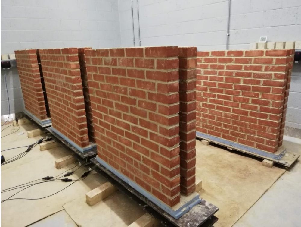
Figure 3: Six wall specimens in the curing room, being cured for six months. The double set of plates with interposed loadcells can be seen under the first row of walls. Each specimen is built on insulating material to prevent temperature bridges from the plates
