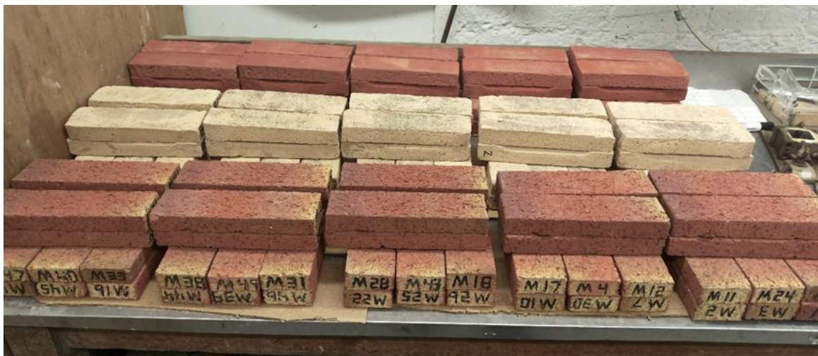
Figure 3: b) Specimens grouped by similar thickness in 5 batches for the three brick types, ready for bonding
