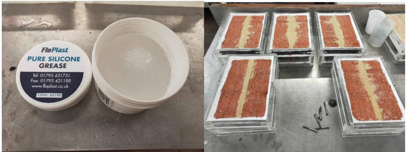
Figure 12: Silicone grease and fully assembled box sets, before tightening with screws
