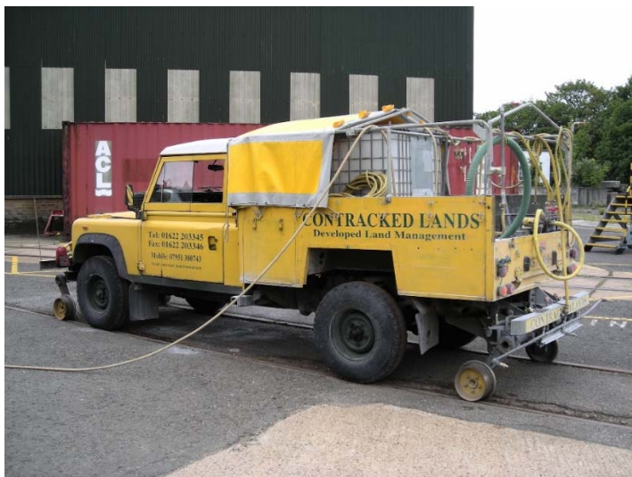
Figure 6.6 Road/Rail Landrover weedkilling sprayer
