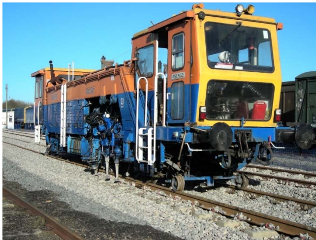
Figure 6.3 Main line tamping machine
