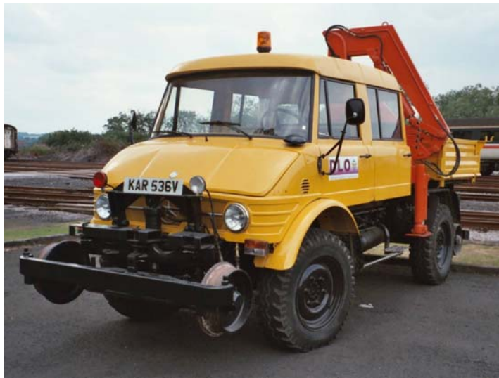
Figure 6.5 Road/Rail Unimog load carrier with crane arm
