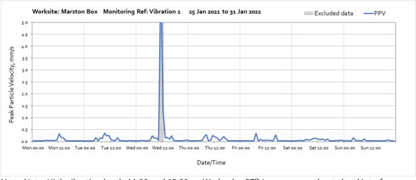
Note: Note: High vibration levels 11:00 and 13:00 on Wednsday 27<sup>th</sup> January were due to local interference and are not representative of HS2 vibration levels.
