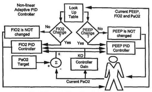
Figure 2. Components of the non-linear adaptive PID controller.
