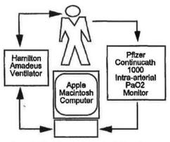
Figure 1. Hardware components of closed-loop control system.
