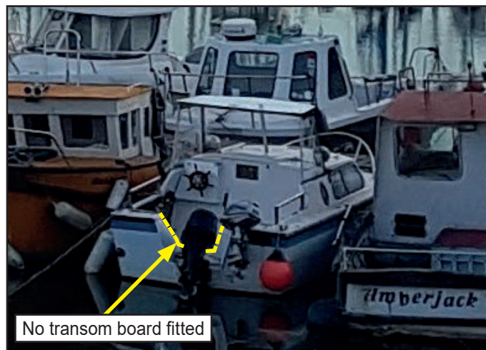
Figure 3: James 2 - showing low freeboard in way of the outboard motor
