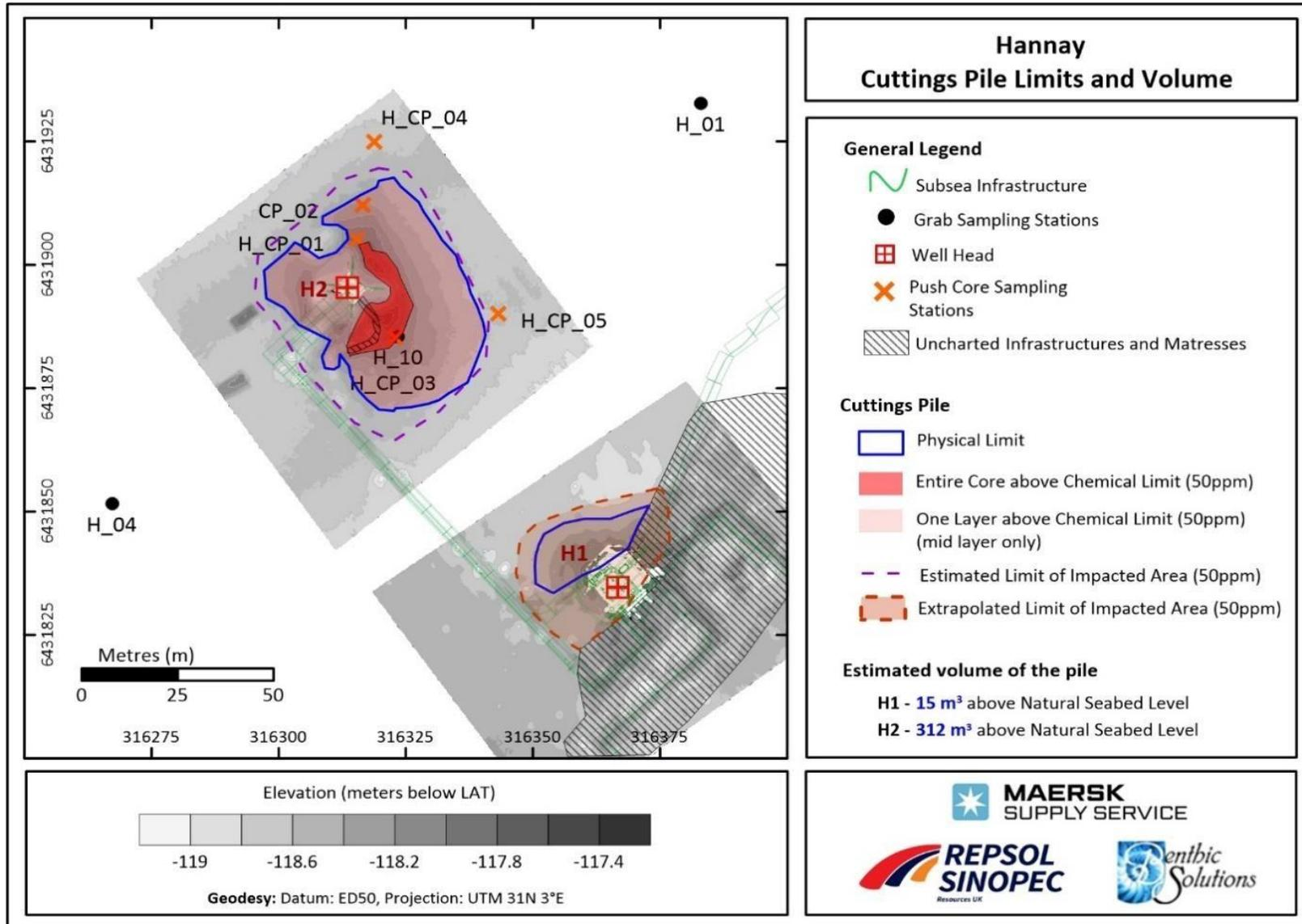
Figure 5-6: Estimated limit and volume of the cuttings at the Hannay wells (Benthic Solutions Ltd., 2019a).
