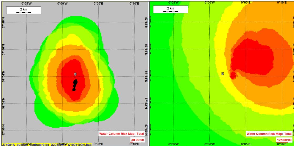
Figure 8-8: Risk to the water column at day 3 (left, 0.0066 km<sup>3</sup>) and at day 12 (right, 0 km<sup>3</sup>).
