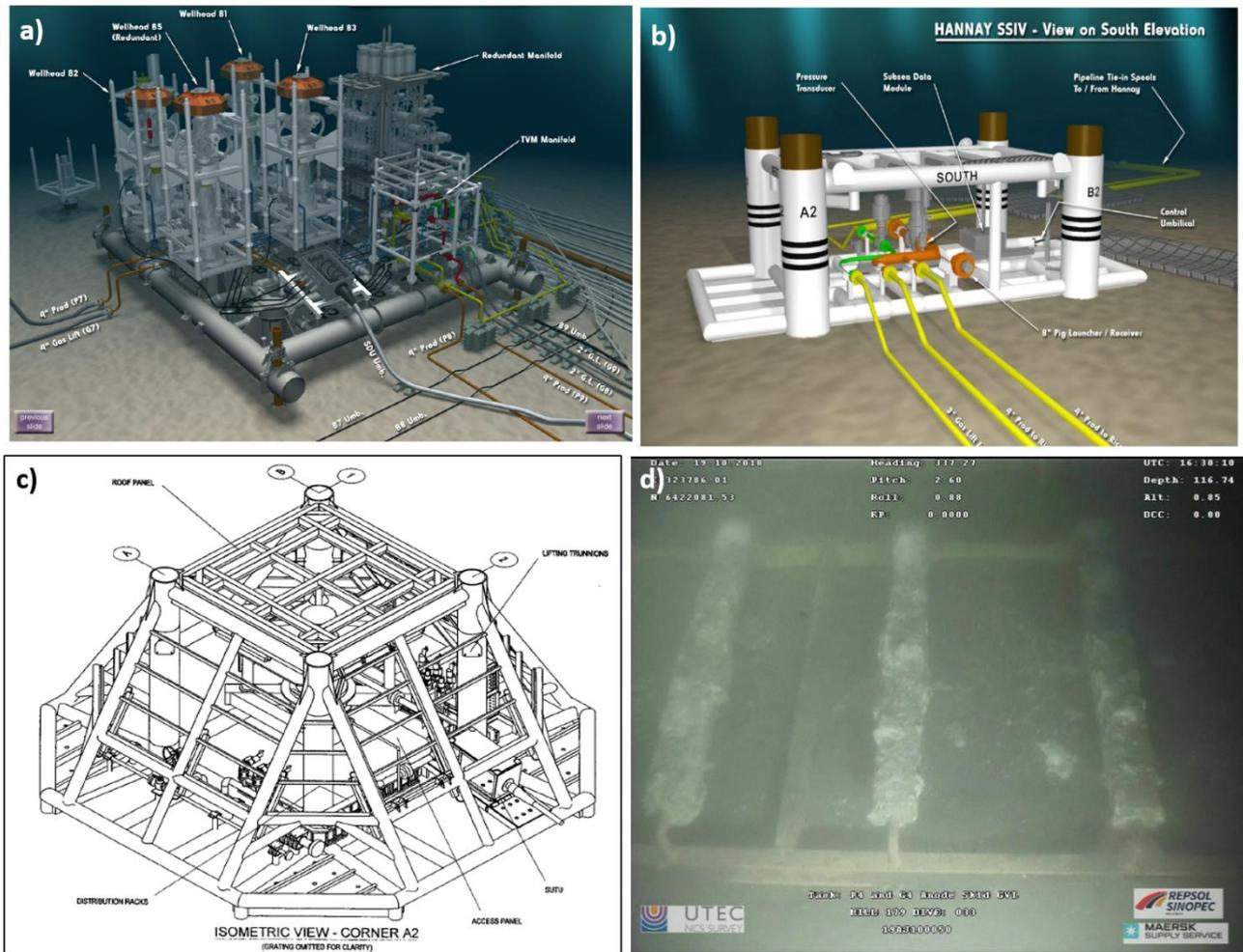
Figure 3-3: Schematics / photographs of some of the Buchan and Hannay subsea structures: a) Buchan template; b) Hannay SSIV; c) integrated manifold/WHPS and d) anode skid.
