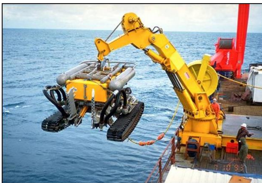
Figure 10: Example Jetting/Trenching Unit
