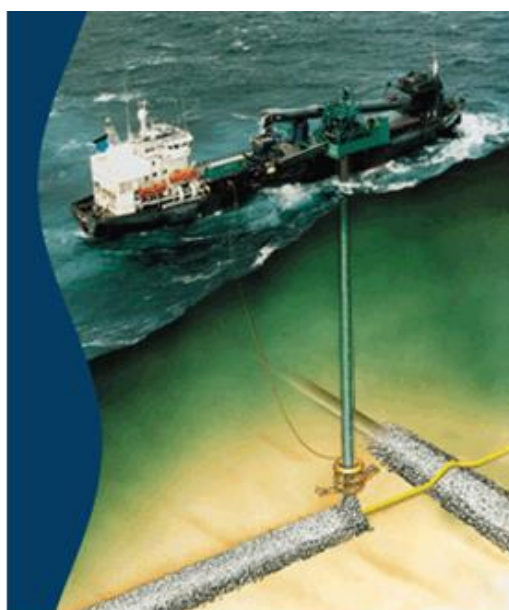
Figure 9: Typical Rock Dumping Activity
