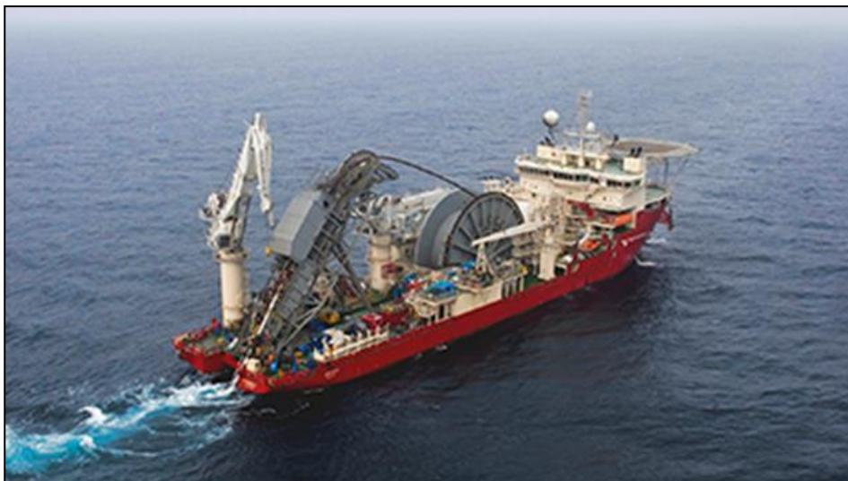
Figure 3: Typical Reel Lay Vessel
