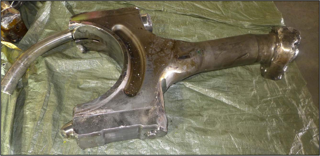
Figure 19: Section of A5 connecting rod (after removal from engine room)
