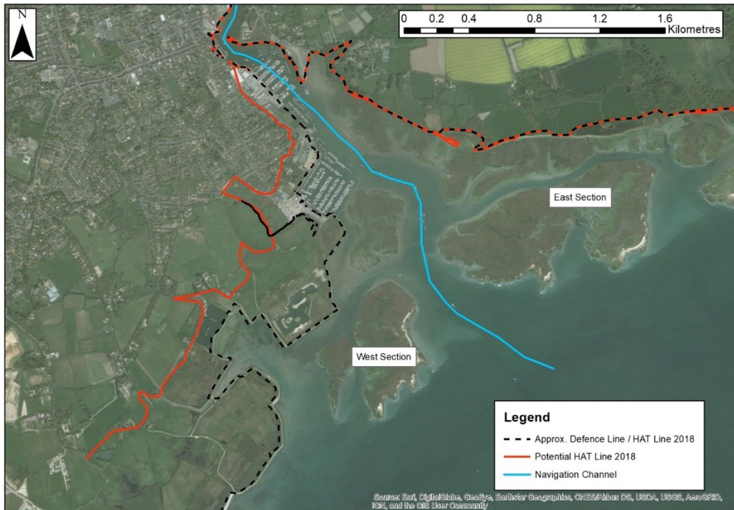
Figure 0.2: Aerial image of site with dashed line indicating present defence line and HAT from AIMS data and red line indicating potential present day HAT line in the absence of defences.
