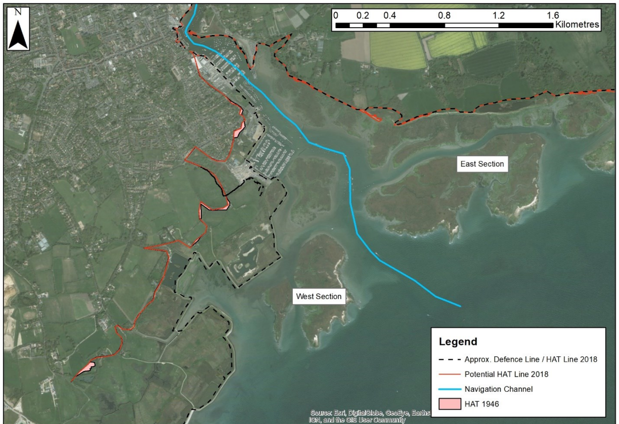
Figure 0.4: Differences in area between 1946 HAT (shown in pink) and 2018 HAT line (blue) in the absence of defences.
