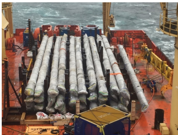
PL5 Spool Sections Recovered to CSV (Asbestos Precautions Visible)
