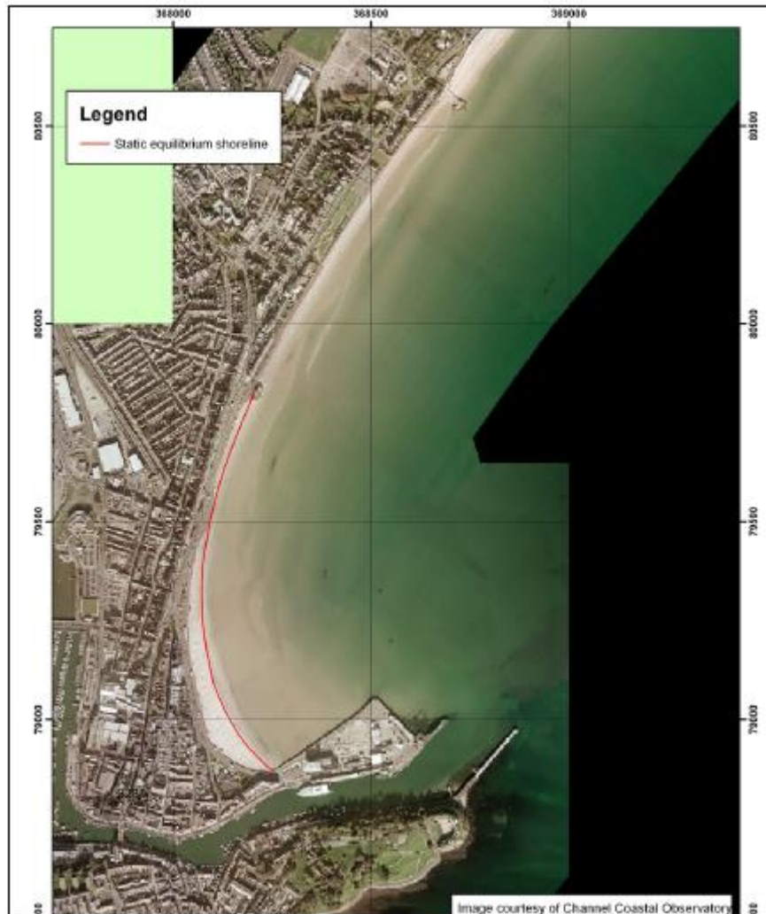
Figure 4.6 Output from application of the equilibrium parabolic bay planshape equation to Weymouth Bay
