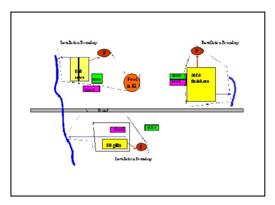
Manure and/or slurry from all houses is stored at the point of production. Surface water from roofs and clean yard drainage is discharged to the river via a soakaway, at each group of houses. Contaminated yard drainage at each group of houses is directed to individual holding tanks and then spread to land.
