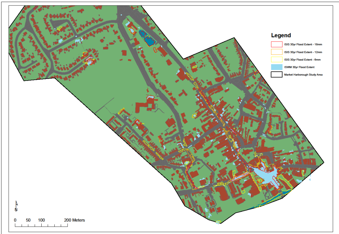
Figure 2.1 Comparison of flood extents for Market Harborough, southern area, 1 in 30 storm event
