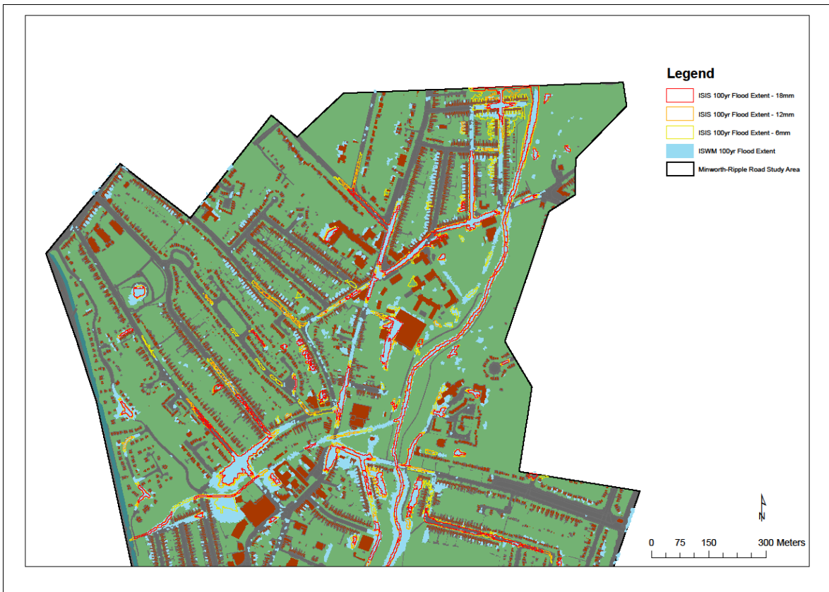
Figure 2.3 Comparison of flood extents for Stirchley, northern area, 1 in 100 storm event
