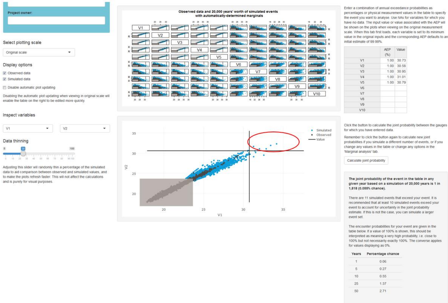
Figure 4.2 Joint probability results for the validation case study where a 1% chance has been applied to all 5 AD variables
