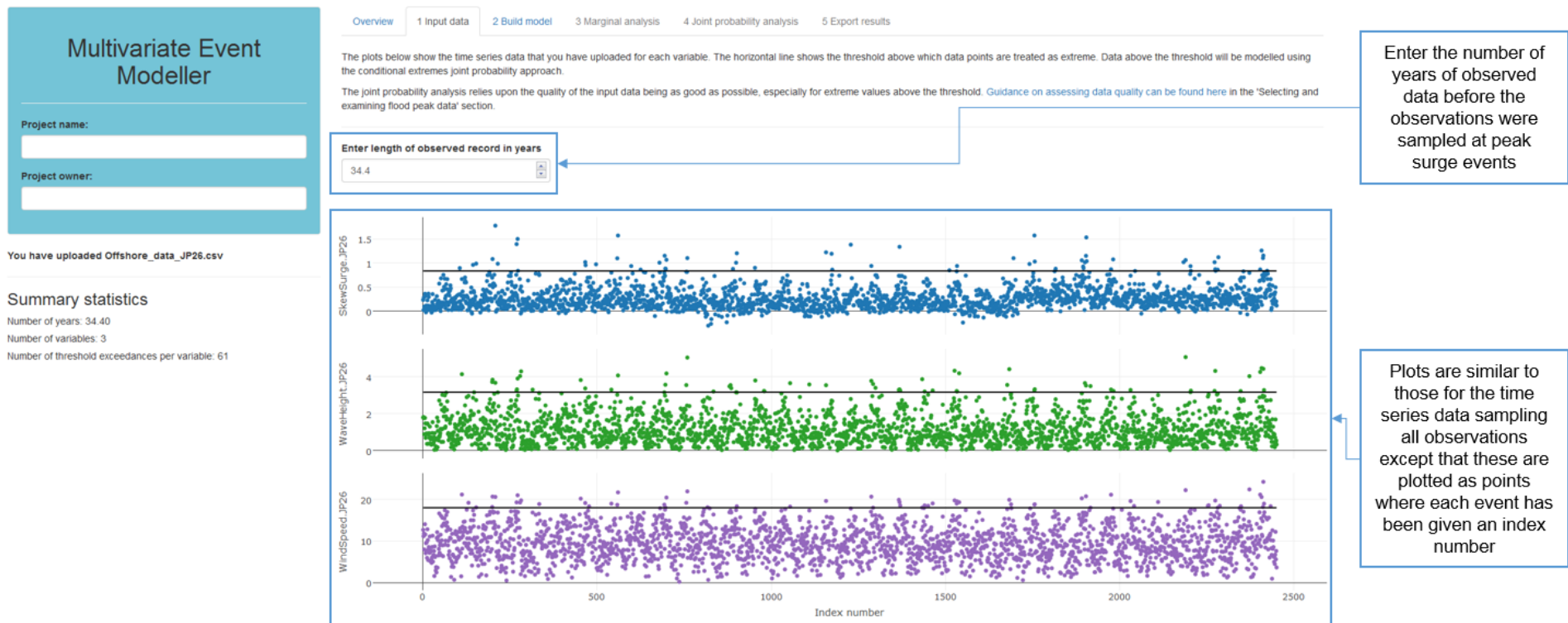
Figure 3.5 'Input data' tab after observations sampled at peak surge events (or a saved model which used this type of data) have been uploaded
