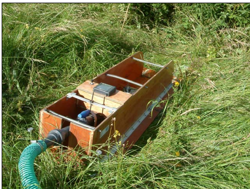
Figure 1.1 Erosion measurement device (EMD) used to test the erodibility of test areas on the floodbanks.
