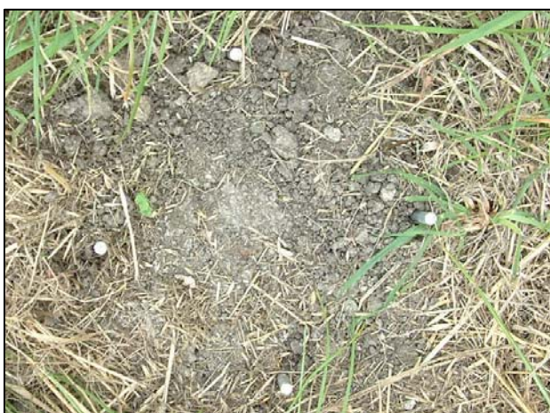
Figure 2.1 Test area marked out by the four marker pins which provide reference points for the recording of the profiles before and after the test.
