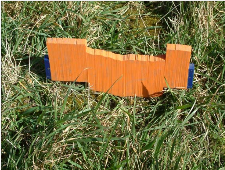
Figure 2.2 'Vitrex' plastic profile gauge used to record the profiles of each erosion plot before and after the test.
