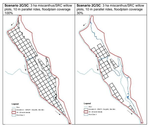
Figure 3.2 Modelled scenario configurations for Severn at Uckinghall<sup>1</sup>
