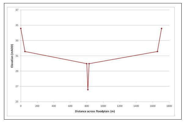
Figure 3.5 Theoretical model river cross-section
