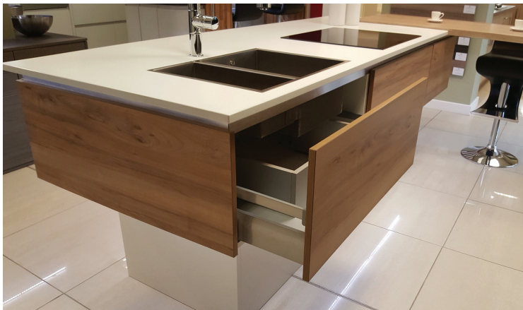
Raised island. Built in hobs and ovens can be raised above the likely flood level
